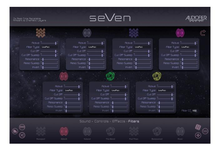
The **Filters Page** offers various parameters for customizing your filter. You can select a filter type, adjust its cutoff frequency and resonance, and even assign its behavior to the mod wheel or a user-defined MIDI CC.
